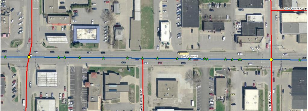
Figure 11: Access points between two signalized intersections on Lincoln Way in Ames, Iowa
